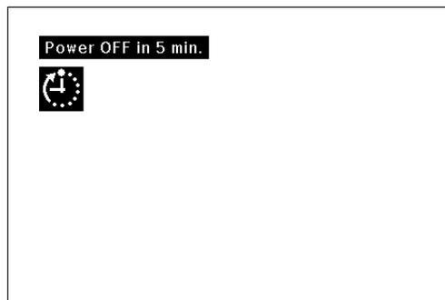
When no input signal is detected for more than 15 minutes, the projector will automatically shut down. The on-screen message on the left will appear five minutes before the power is automatically turned off.
