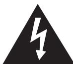
The lightning flash with arrowhead symbol, within an equilateral triangle, is intended to alert the user to the presence of uninsulated "dangerous voltage" within the product's enclosure that may be of sufficient magnitude to constitute a risk or electric shock to persons.
