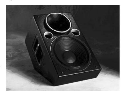
The compact speaker system shall be of the two-way type, with a 12" lowfrequency loudspeaker front-mounted in a ducted bass-reflex hardwood plywood enclosure, a compression driver mounted on a high-frequency horn which has a 1.4" throat, and a separate Control Electronics Unit.
