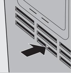
**14** Press the filter reset button with a thin tool.
