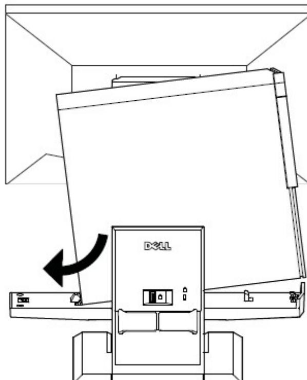
**4** Ensure the computer chassis is seated on both ends of the AIO stand.
