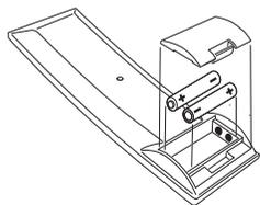
Remove the back cover to reveal the battery compartment and make sure the batteries are inserted the right way round.
