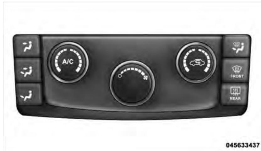
The Dual-Zone Manual Climate Controls allow both driver and front passenger seat occupants to select individual comfort settings. The controls consist of a series of outer rotary dials and inner push knobs.
