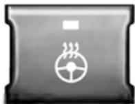
Press the switch to turn on the heated steering wheel. The light on the switch will illuminate to indicate the steering wheel heater is on. Pressing the switch a second time will turn off the heated steering wheel and light indicator.
