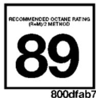
This engine is designed to meet all emissions regulations and provide satisfactory fuel economy and performance when using high-quality unleaded gasoline having an octane range of 87 to 89. The manufacturer recommends the use of 89 octane for
