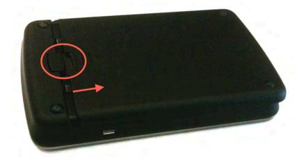
2 Insert your fingernail into the battery removal divot and lift the battery out of the battery compartment.
