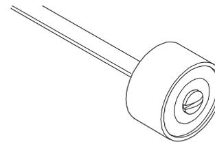
**Sanding band shanks:** Sanding band shanks feature an expanding core that hold disposable bands securely. To contract the core to remove or install a band, loosen the screw. Tightening the screw expands the core.
