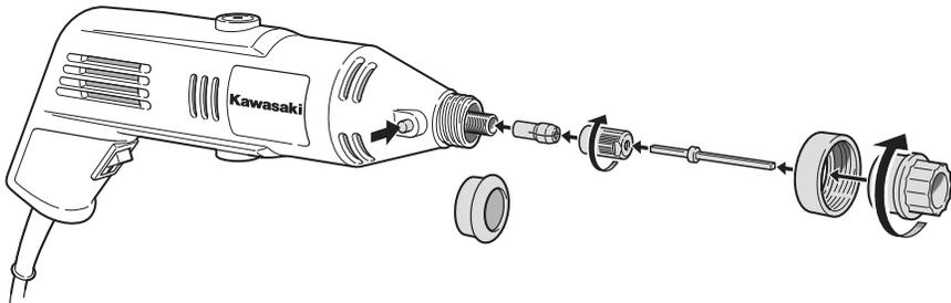
1. Remove spindle nut from the tool by turning it counterclockwise.
