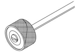
**Brushes:** Wire brushes are useful for cleaning and polishing metal, while bristle brushes are suitable for cleaning softer surfaces. As with all rotary tool accessories, you should let the speed do the work without applying excessive force. Use the bristle tips only without mashing the brush against the work piece as shown in the top part of the illustration on the right.
