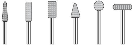
**Grinding stones:** Use these stones for smoothing hard materials such as wood, plastic, and metal. Be sure not to allow the work piece to overheat as this can cause charring (wood), melting (plastic), or discoloration (metal). Aluminum oxide (red) accessories are best for wood, metals, and plastics, while silicon carbide (blue) accessories are best for very hard surfaces such as glass.
