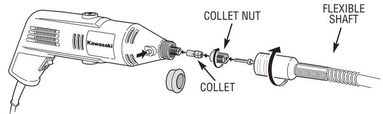
**⚠ WARNING** Never bend the flexible shaft with a radius of less than 6" when operating. Please store the flexible shaft in the designated compartment of the tool box when not in use.
