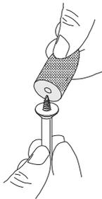
**Polishing wheels:** These accessories are useful for removing tarnish and weathering on metal and for polishing plastics. They require a special shank with a screw tip. To prepare a polishing wheel, screw the felt onto the shank tip. Reverse to remove. Polishing grease can be used in small quantities to aid in polishing metal. Lower speeds are best for these accessories.
