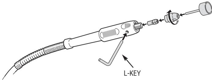
To change the collet or install an accessory in the flexible shaft, follow the same general procedure as for changing the collet and for installing accessories on the rotary tool. To lock the spindle, rotate the collet until the hole in the shaft is aligned with the hole in the flexible collar. Insert the L-key through the holes to lock the shaft.
