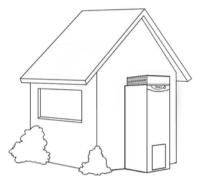
The water heater must not be installed in an area with a corrosive atmosphere where chemicals are stored or where aerosol propellants are released. Remember the air may be safe to breathe, but when it goes through a flame, chemical changes take place which may attack the water heater.
