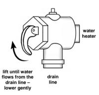
The temperature pressure relief valve should be checked for performance or replaced at intervals not exceeding 5 years, or more frequently in areas where there is a high incidence of water deposits (refer to "Water Supplies" on page 30).
