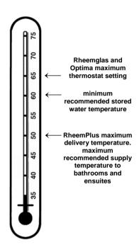
We recommend and it may also be required by regulations that an approved temperature limiting device be fitted into the hot water pipe work to the bathroom and ensuite when a Rheemglas or Optima water heater is installed. This will keep the water temperature below 50°C at the bathroom and ensuite. The risk of scald injury will be reduced and still allow hotter water to the kitchen and laundry.
