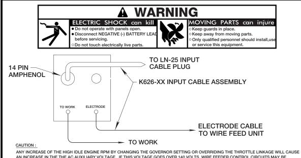
AN INCREASE IN THE THE AC AUXILIARY VOLTAGE. IF THIS VOLTAGE GOES OVER 140 VOLTS, WIRE FEEDER CONTROL CIRCUITS MAY BE DAMAGED. THE ENGINE GOVERNOR SETTING IS PRE-SET AT THE FACTORY - DO NOT ADJUST ABOVE RPM SPECIFICATIONS LISTED IN THE ENGINE WELDER OPERATING MANUAL.
