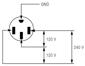
matic idle feature is in both legs of the three wire circuit as shown below.
