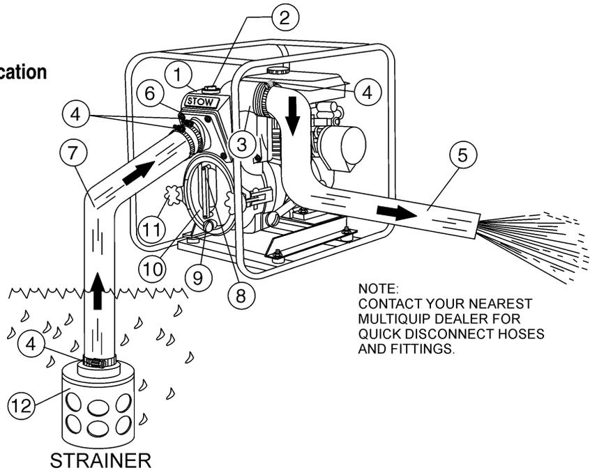
1. **Pump** – The STOW Model T-20H is 2-inch trash pump used in general de-watering applications. Typical dewatering applications consist of manholes, septic tanks, fast and slow seepage ditch water, silt water, mud water and muck water.
