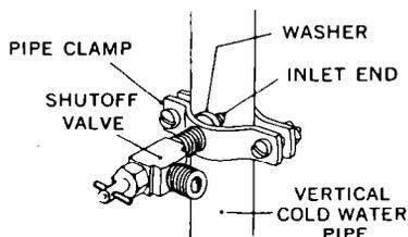
**D6.** Slip *compression nut* and *compression sleeve* on copper tubing as shown in diagram. Insert end of tubing into *outlet end* squarely as far as it will go. Screw *compression nut* to *outlet end* with adjustable wrench. Do not overtighten. Turn ON main water supply and flush out tubing until water is clear. Turn OFF *shutoff valve* on the water pipe. You are now ready to connect other end of  $\frac{1}{4}$ -inch copper tubing to inlet tube or water valve on back of refrigerator.
