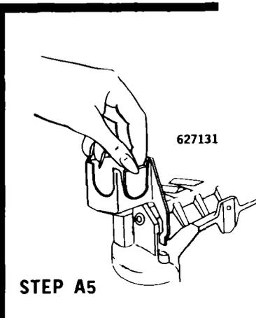
**A5.** Be sure the sliding adapter plug (#627131) is in the side of the water fill trough as shown.
