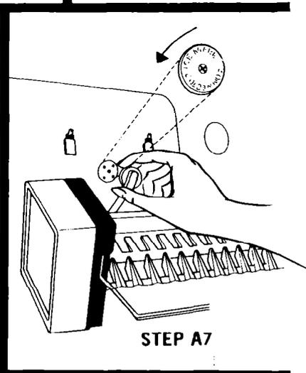
**A7.** Remove ICE MAKER CONNECTOR plug cover by inserting screw driver in slot and rotating driver to left. Insert Ice Maker connector into the receptacle under "ICE MAKER CONNECTOR" plug cover.
