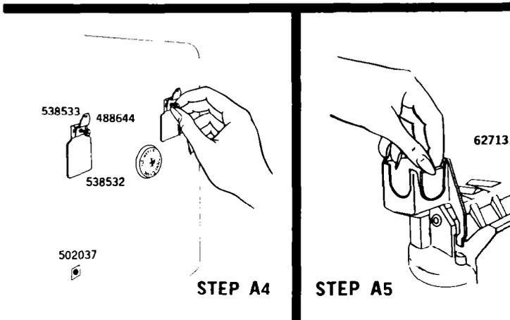
**A4.** Insert the 2 brackets (#538532) into the side of the freezer wall. Attach one clip (#538533) and screw (#488644) to each of the two brackets. Leave screw loose. Insert grommet (#502037) into square hole on left wall.
