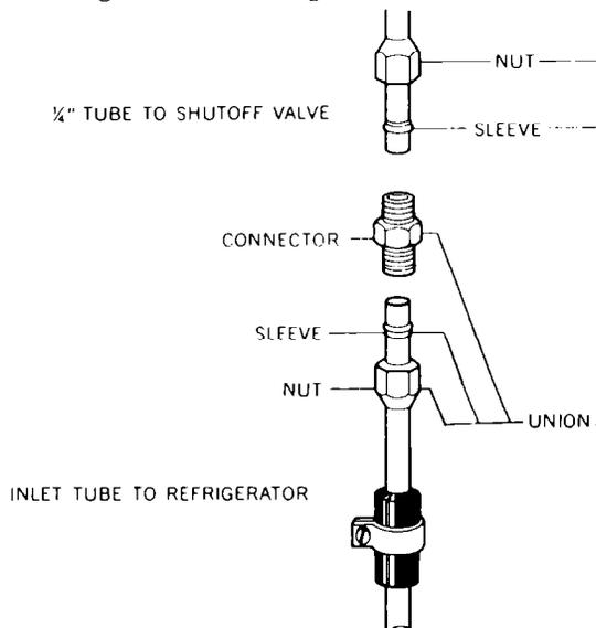
**D8.** Turn shutoff valve on. **TIGHTEN ANY CONNECTIONS OR NUTS THAT LEAK.**
