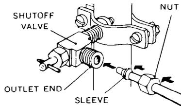
**D7.** Assemble *compression nuts* on tubing as shown in diagram. Insert ends of tubing into *connector* and tighten *compression nuts*. Be sure ends of tubing are squarely in connector as far as they will go. Do not overtighten.
