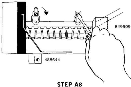
**A8.** Attach the Ice Maker to the side of the freezer by inserting screw (#488644) through bracket on bottom front of Ice Maker, and into grommet (#502037). Rotate clips down and tighten screws. Be sure that water fill tube (#849909) is in water fill trough of Ice Maker as shown in A8.
