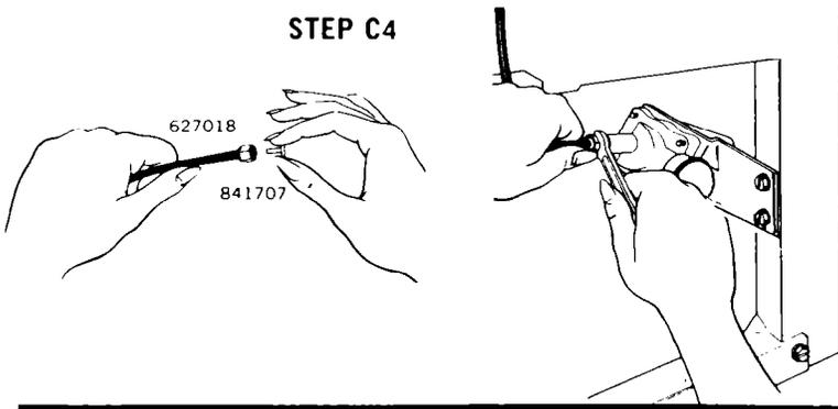
**C4.** Slide nut and sleeve (#627018) over tubing. Push tube insert (#841707) into end of tubing. Push end of tubing into water valve. Tighten the retaining nut, but do not overtighten.
