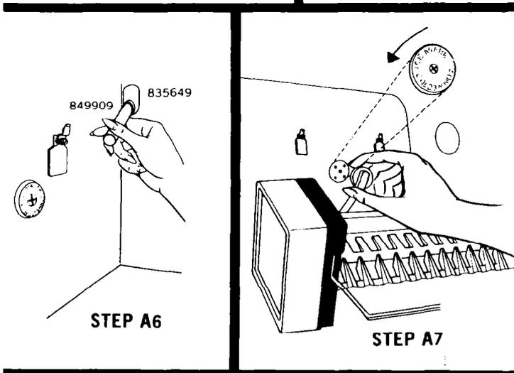
**A6.** Remove (#849909) aluminum fill tube from package. Cut off tube as shown on instructions for top freezer models packed with tube. Slip #849909 up over water inlet tube (factory installed). Make sure that tubes are properly engaged by looking in oblong hole. Move grommet (#835649) up over tube to cover oblong hole.
