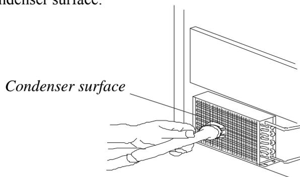
5. Remove dirt and lint from the condenser fins and the unit compartment with a brush attachment on a vacuum cleaner.
