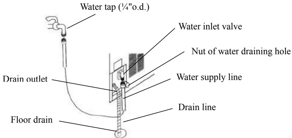
*NOTE: Connection to the water line may vary according to installation requirements.*
