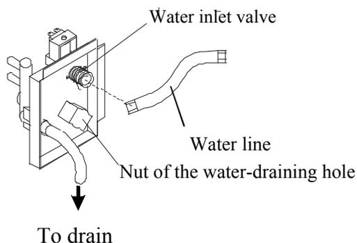
Minerals that are removed from water during the freezing cycle will eventually form a hard scaly deposit in the water system. Cleaning the system regularly helps remove the mineral scale buildup. How often you need to clean the system depends upon how hard your water is or how effective your filtration may be. With hard water of 15 to 20 grains/gal. (4 to 5 grains/liter), you may need to clean the system as often as every 6 months.
