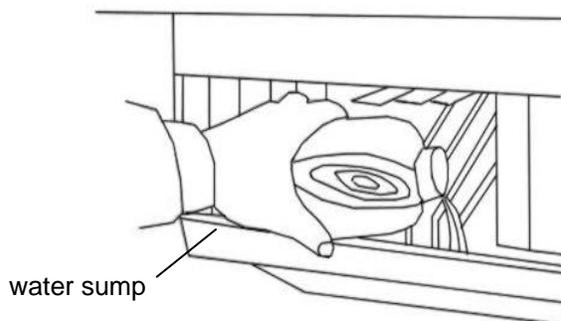
5. Allow 30 minutes for proper cleaning. After cleaning, shut off the power switch, and unscrew the nut of the water-draining hole on the rear of the unit. Drain off the waste water to some container, and then screw the nut on tightly when the waste water is fully drained off.
