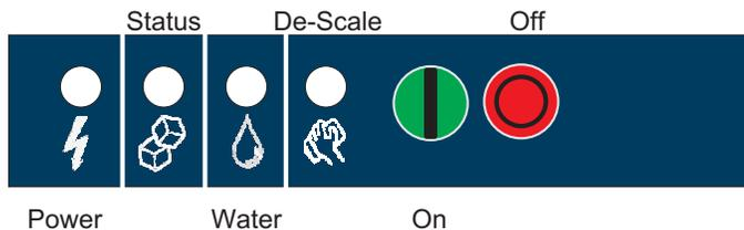
To switch the machine OFF, push and release the Off button. The machine will shut off at the end of the next cycle.
