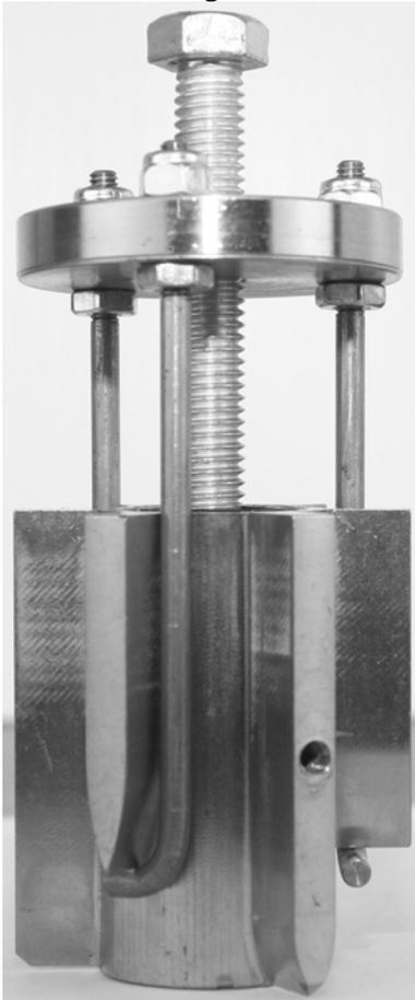
8. Install new cutter head and secure with three bolts removed in step 7. Use removable loctite on bolt threads.
