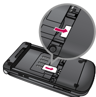
To insert the SIM card
