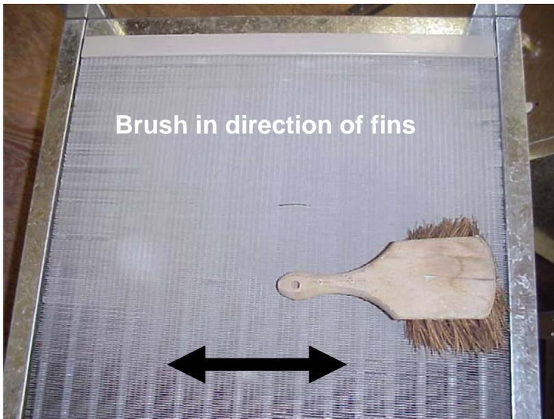
At 6 month intervals the fins on the inlet side of the condenser (bottom as shown) should be brushed free of dust and dirt. Brush in the direction of the fins as noted by the arrows.
