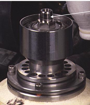
4. Unscrewing the auger stud
