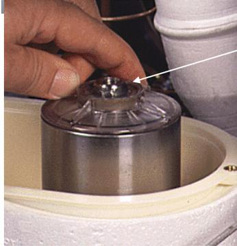
3. Removing the water shed and unscrewing the breaker cover.
