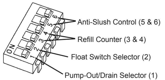
\* Functions of S2 dip switch nos. 2 through 6 depend on program version.
