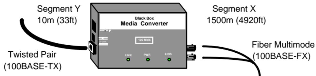
**Connectivity between 100BASE-TX and 100BASE-FX Ethernet Media.**
