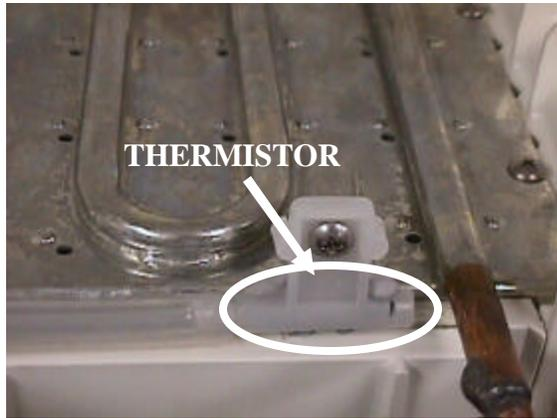
The AM series uses a combination thermistor and control board to control the sequence of operation. When the toggle switch is placed in the “ON” position and the bin control calls for ice, the unit will begin in the initial harvest cycle. Starting the unit in harvest allows the compressor to start in an unloaded condition, greatly extending the life of the compressor. This operation is common among all Hoshizaki cube icemakers.
