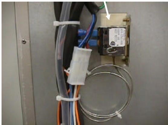
The AM series uses a thermostatic bin control located on the right rear side of the ice storage compartment. This control will open when ice touches the sensing bulb and the unit will shut down
