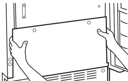
4. Remove dirt and lint from the condenser fins and the unit compartment with a brush attachment attached to a vacuum cleaner.
