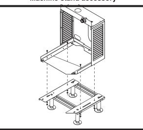
Mount louvered docking assembly to machine stand accessory
