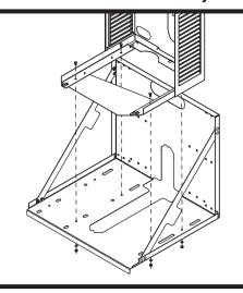
Mount louvered docking assembly to wall bracket accessory
