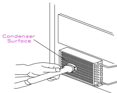
4. Remove dirt and lint condenser fins and the unit compartment with a brush attachment on a vacuum cleaner.
