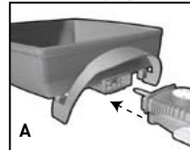
1. Make sure the variable temperature control is set to "Min". Insert the probe firmly into the socket found at the side of the appliance (A).
