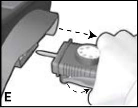
9. To use skillet for table service, unplug appliance. To remove the variable temperature control probe, hold the cool-touch handle on the side of the skillet. Press the quick-release lever and pull out the control **(E)**.
