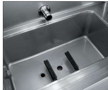
Pressed tanks in the pre-wash, wash and rinse zones, sloped towards drain to prevent dirt build up.
