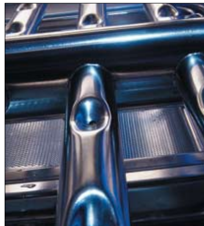
The Maximum Water Contact (MWC) wash arms are positioned along the full length of the wash tank to wash in the shortest possible space. Thus doubling the amount of wash water contact time in comparison to the traditional wash arm configurations. Just because a basket is in the wash zone for 2 minutes, it doesn't mean it is being washed in water for 2 minutes.
