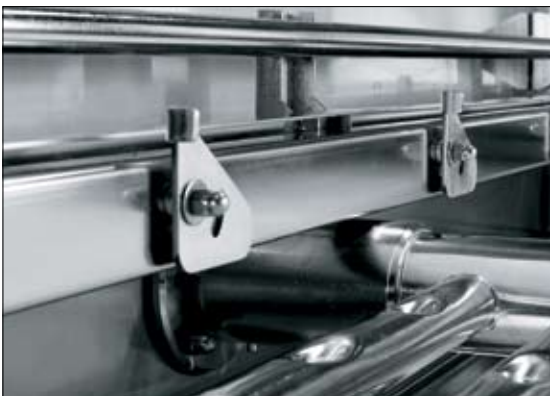
Feeding system fingers are more resistant thanks to their stainless steel construction.
