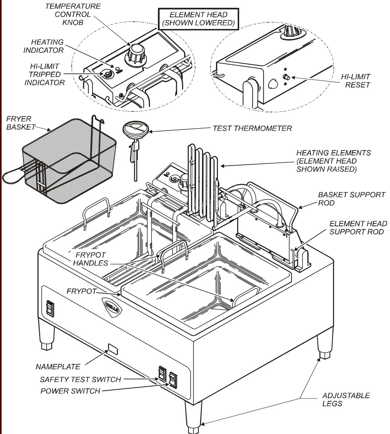
Fig. 1 Countertop Fryer with Safety Test System™ Features & Operating Controls
