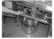
16. Replace the emptied stock pot below the drain manifold opening, and repeat steps 14 and 15 as many times as needed.
