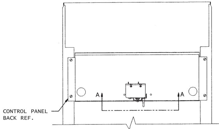
LINE UP TEMPLATE ON EXISTING HOLE AS SHOWN.
