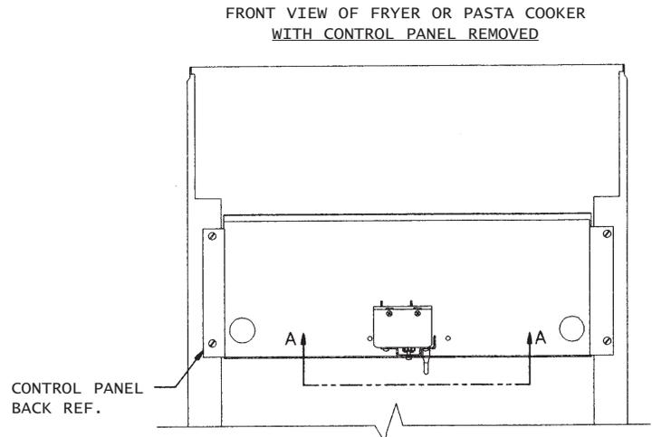
LINE UP TEMPLATE ON EXISTING HOLE AS SHOWN.
