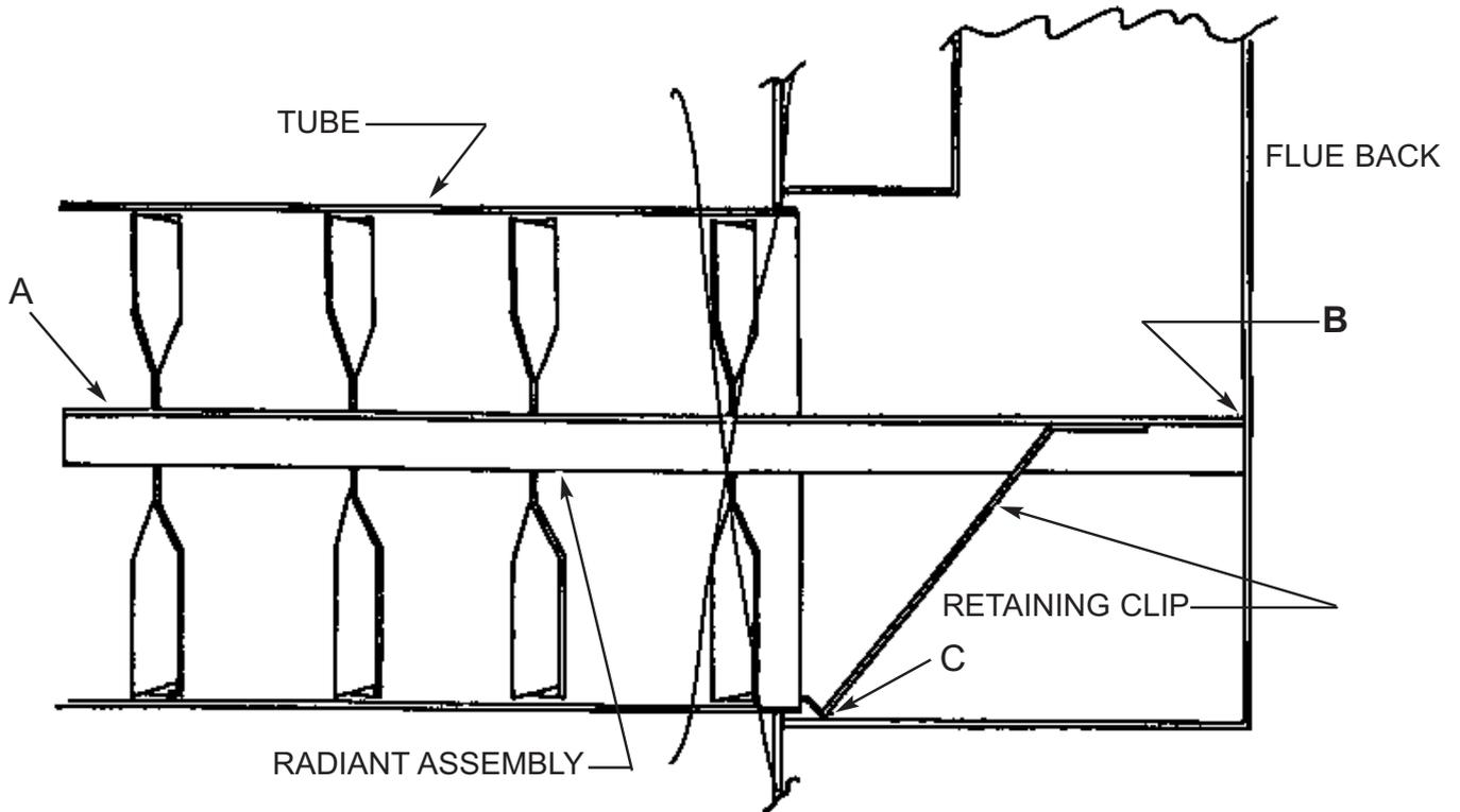
1. To remove radiant assembly remove the burners from the manifold then grip the end of the radiant angle bar at point "A" and pull forward and out of the tube.
