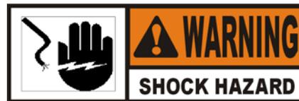
This fryer **must** be adequately and safely grounded (earthed) or electrical shock could result. Refer to local electrical codes for correct grounding (earthing) procedures or in absence of local codes, with The National Electrical Code, ANSI/NFPA No. 70-(the current edition). In Canada, all electrical connections are to be made in accordance with CSA C22.1, Canadian Electrical Code Part 1, and/or local codes.
