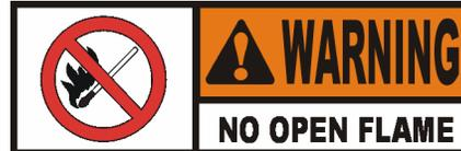
To avoid fire or explosion, never use a lighted match or open flame to test for gas leaks. Ignited gas could result in severe personal injury and/or property damage.
