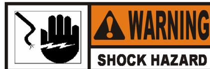
To avoid electrical shock, this appliance must be equipped with an external circuit breaker which will disconnect all ungrounded (unearthed) conductors. The main power switch on this appliance does not disconnect all line conductors.
