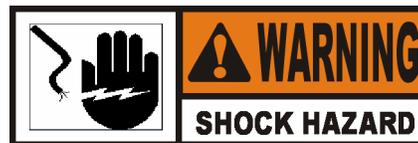
To avoid electrical shock, this appliance must be equipped with an external circuit breaker which will disconnect all ungrounded (unearthed) conductors. The main power switch on this appliance does not disconnect all line conductors.
