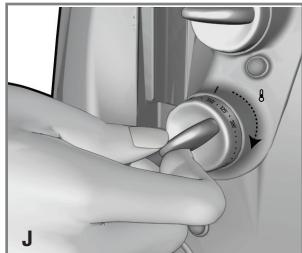
2. While appliance is heating the thermostat light will be off. The light will turn back on when the selected temperature has been reached (**J**).
