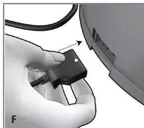
7. This fryer has a detachable cord with a magnetic power attachment to be inserted to the rear of the fryer. This must be inserted with the white dot facing upward (**F**).
