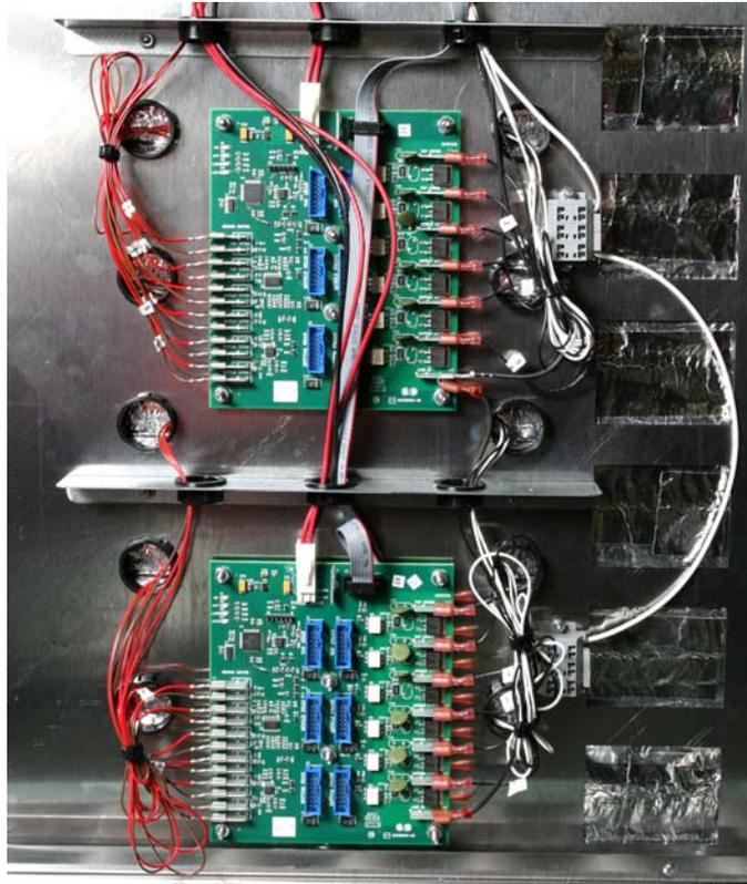
**Fig. 6:** Distribution board shown with display cables removed.
