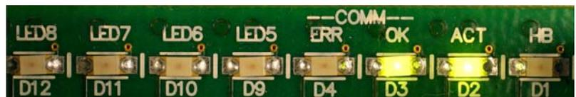
Fig. 4: Master Control Board LED's
