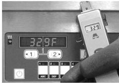
If the two temperatures are less than 5°F (3°C) apart (either plus or minus), you do not need to adjust the temperature setting.
