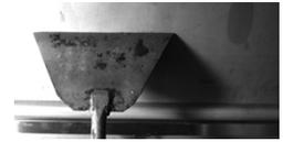
On an electric fryer, next use the putty knife to scrape all soft grease and hard carbon from all sheet metal around the fryer, the standoff piece, and the fryer stand. Skip to step 8 after these areas are cleaned.
