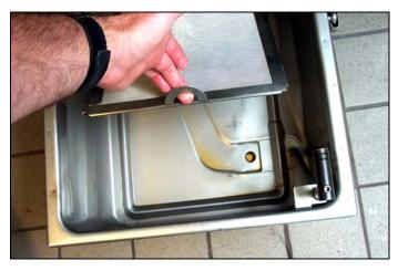
Remove the crumb screen and filter assembly from the pan. Clean all components with a solution of detergent and hot water, then dry thoroughly.
