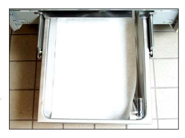
Lay a sheet of filter paper or a filter pad over the screen. <u>If using the PAD</u>, <u>ensure the rough side of the pad is up.</u>
