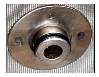
Inspect the filter screen O-ring.
