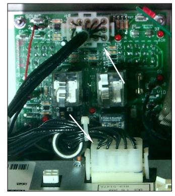
If replacing harness, disconnect the harness from the controller and interface board (arrows).
