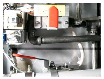
Rotate the handle to the left to return oil to the frypot. Rotate to the right on fryers with optional reardischarge to dispose of the oil.
