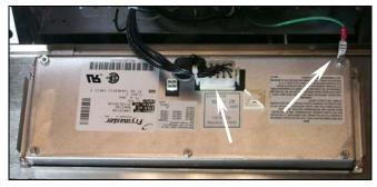
If replacing controller, disconnect the ground wire and the 15-pin connector (arrows).
