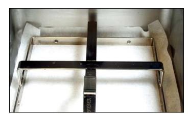
5. Install the hold-down ring over the paper or the pad.
