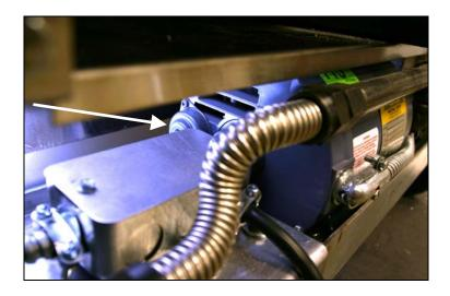
Filter Pump Reset Switch (Arrow)
