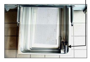
Place the filter screen in the bottom of the filter pan.
