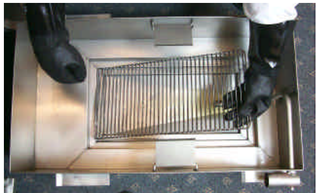
Remove filter screen from filter pan.
