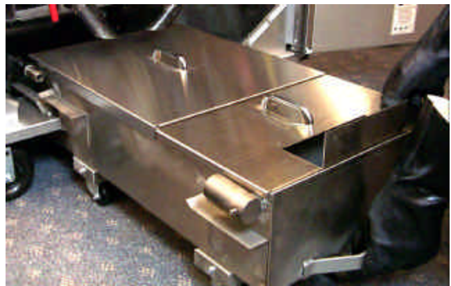
Pushing filter pan back into cabinet. Filter is ready for operation.
