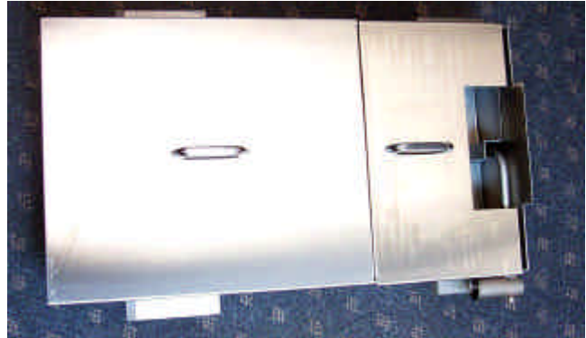
Pan covers properly placed.
