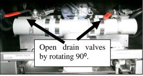
Open the drain valves on the frypot and drain the oil into the filter pan.
