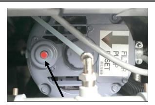
**Filter Pump Reset Switch**
