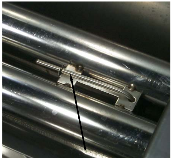
Electronic thermostat probe in frypot (arrow).
