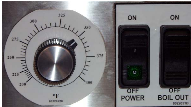
Electronic thermostat controller with power switch and boil-out option.
