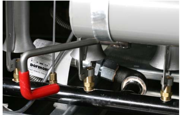
A microswitch is located on the red handle at the drain valve.
