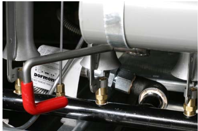
Push the red handle right to open drain valve. Oil will start to drain into filter pan.
