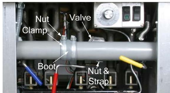
On units with 3" drains, remove the nuts, Teflon tube (not pictured), clamp, boot, and drain tubes. (Step 5.B)
