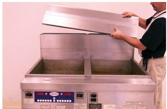
Removing the flue cap.
