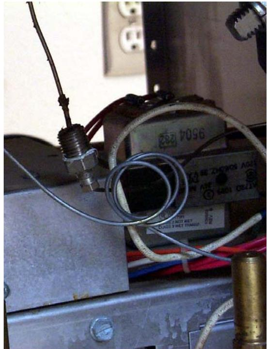
Remove high-limit capillary tube and bulb from the bottom of the frypot.
