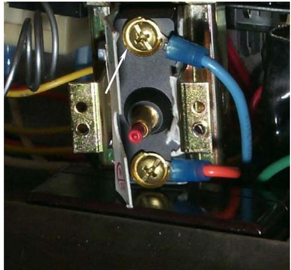
Mark and disconnect high-limit wiring (arrows). Reconnect wires to the same terminals on the replacement high-limit.
