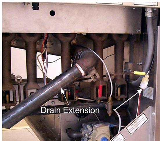
Disconnect the two-pin probe harness connector (arrow). On units with 1.5" drains, remove the drain extension from the elbow on the drain valve.
