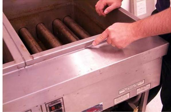
Cutting frypot seal prior to frypot removal.
