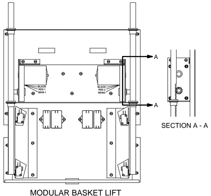
**Binds and jams.** Noisy, jerky, or erratic movement of the lifts is usually due to lack of lubrication of the rods and their bushings. Apply a light coat of Lubriplate or similar lightweight white grease to the rod and bushings to correct the problem.
