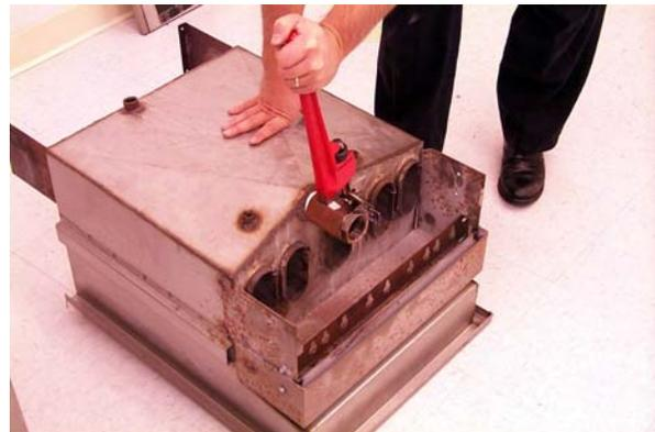
Removing drain valve from frypot.
