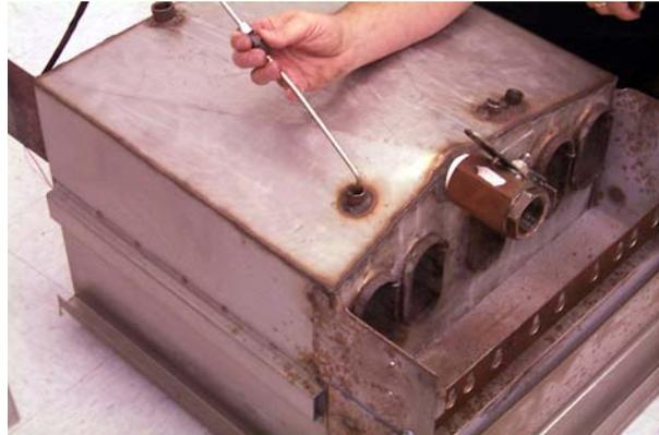
First remove the mounting clips holding the probe in place. Retain mounting hardware for installation of new probe.
