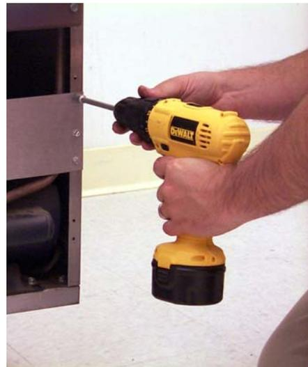
Removing gas manifold shield.
