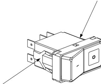
Depress clips on each side to remove switch from control panel.
