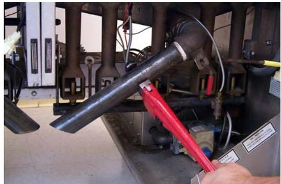
Removing 1.5" drain extension. (Step 19.A)
