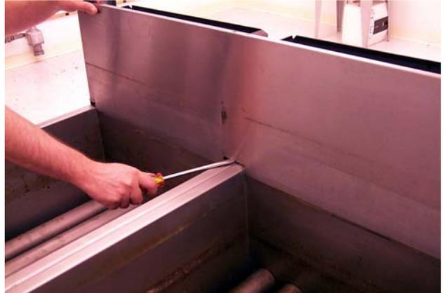
Removing flue cap.
