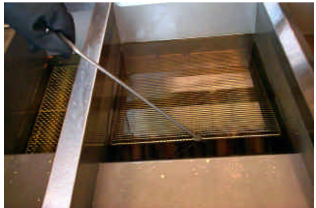
Removing support grid from frypot prior to filtering.
