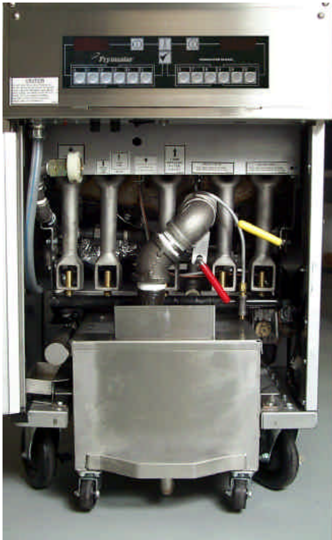
Typical built-in filter installed in a single fryer unit.
