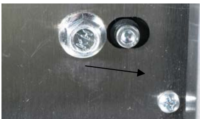
Fig. 8: Loosen the hex bolt and remove the allen screw (arrows, upper photo). Some row positions may have an additional screw securing the bezel to the cabinet (lower photo). Push through the access port (arrow, upper photo), if necessary, to remove the bezel from the cabinet .
