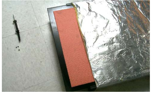
Fig. 12: The heater plate slides from the insulation.
