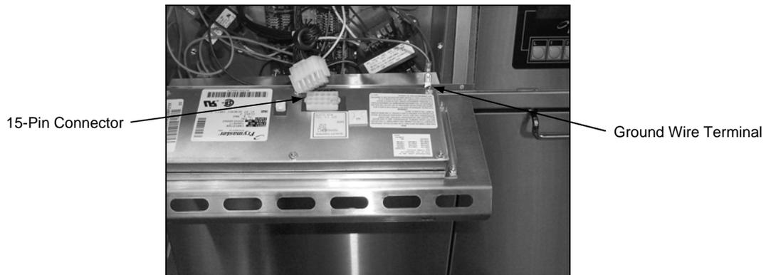
5. Remove the controller from the control panel assembly and install the replacement controller. Reinstall the control panel assembly by reversing Steps 1 and 2.
