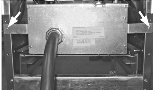
Remove the screws (white arrows) from the tabs on either side of the contactor box.
