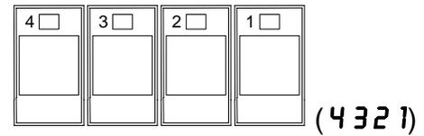
The E-LOG mode is used to view the ten most recent error codes encountered on the fryer. These codes are displayed from 1-10 with the most recent displayed first. The time, date and error code are displayed.
