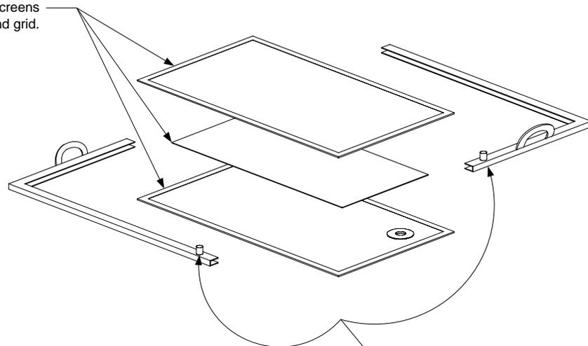
Step 1 - Grasp frame with thumbs on these handles and pull frame apart at corner.
