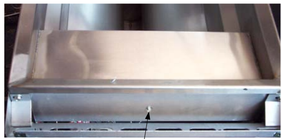
When the topcap is removed, this screw is exposed. It must be removed to free the frypot.
