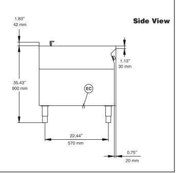
Modular Cooking Range Line S90 Heavy Duty Two Well Electric Deep Fat Fryer, C-Board
