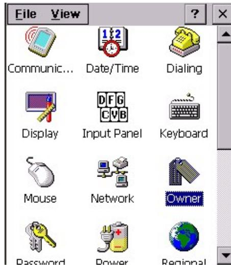
2. Key in the name of the owner, company and the address of the company. Check “Display owner identification”. Tap “OK”. The system will display the owner identification after suspend and power on.
