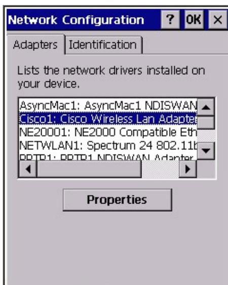
3. Tap “Properties”. Select either obtain IP address via DHCP or specify an IP address.
