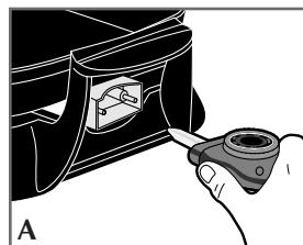
1. Set the temperature control to "Off" and push the probe firmly into the socket on the skillet pan (A). Be sure the control is securely inserted. Always attach the control to the pan FIRST before plugging into an outlet.
