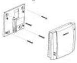
2) Insert the FCT in the wall-mounting bracket
