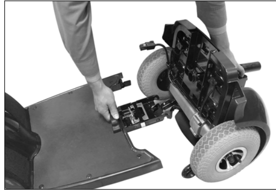
Figure 6. Hold the handle on the floorboard and lift up front section. Front and rear sections can be separated.
